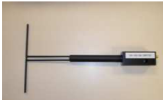
Figure 1 – Satimo COMOSAR Validation Dipole
