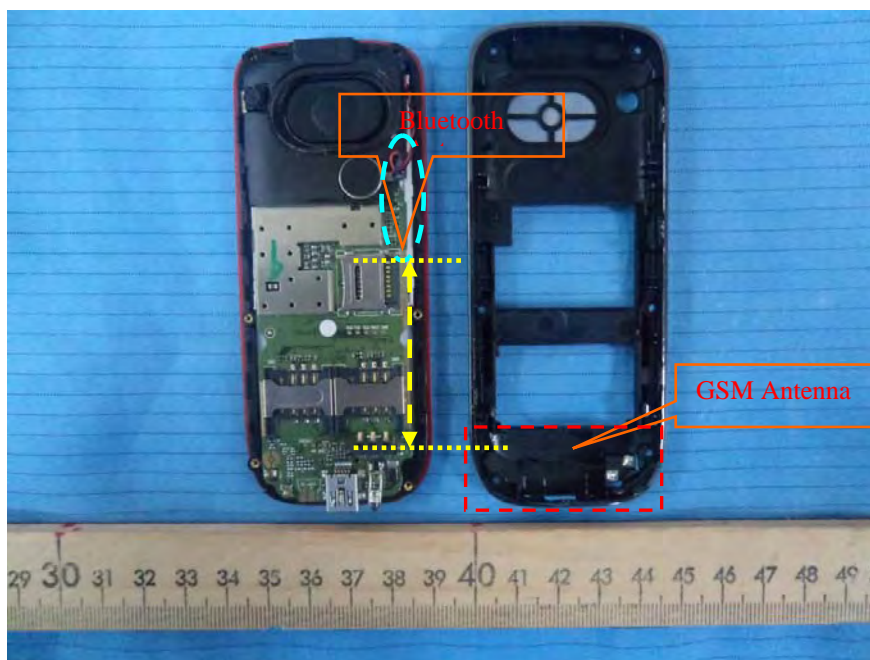
BT and GSM Antenna Location
