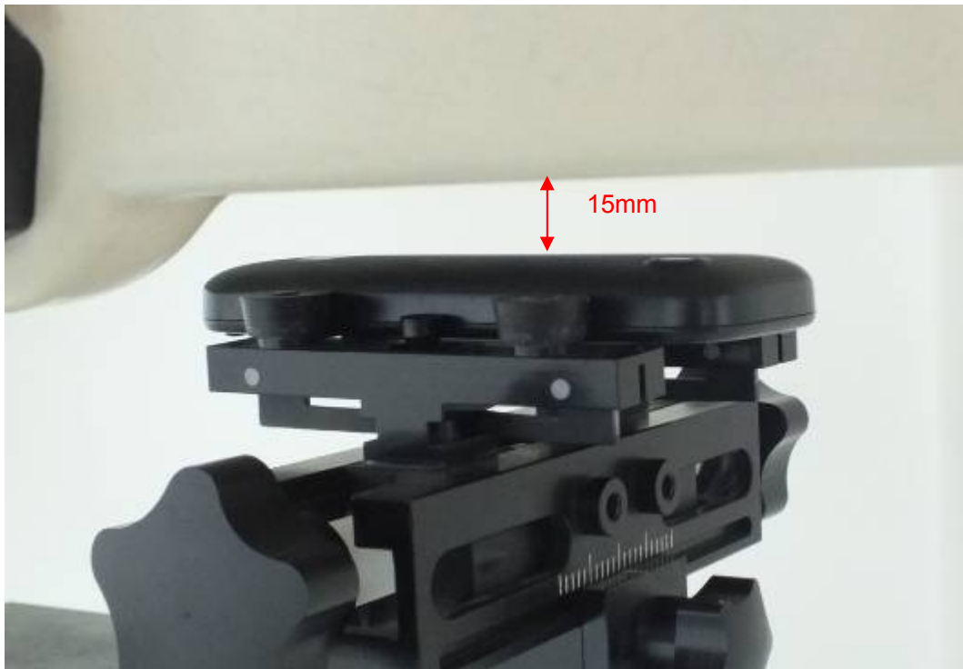
Picture 13: Back Side, the distance from handset to the bottom of the Phantom is 15mm
