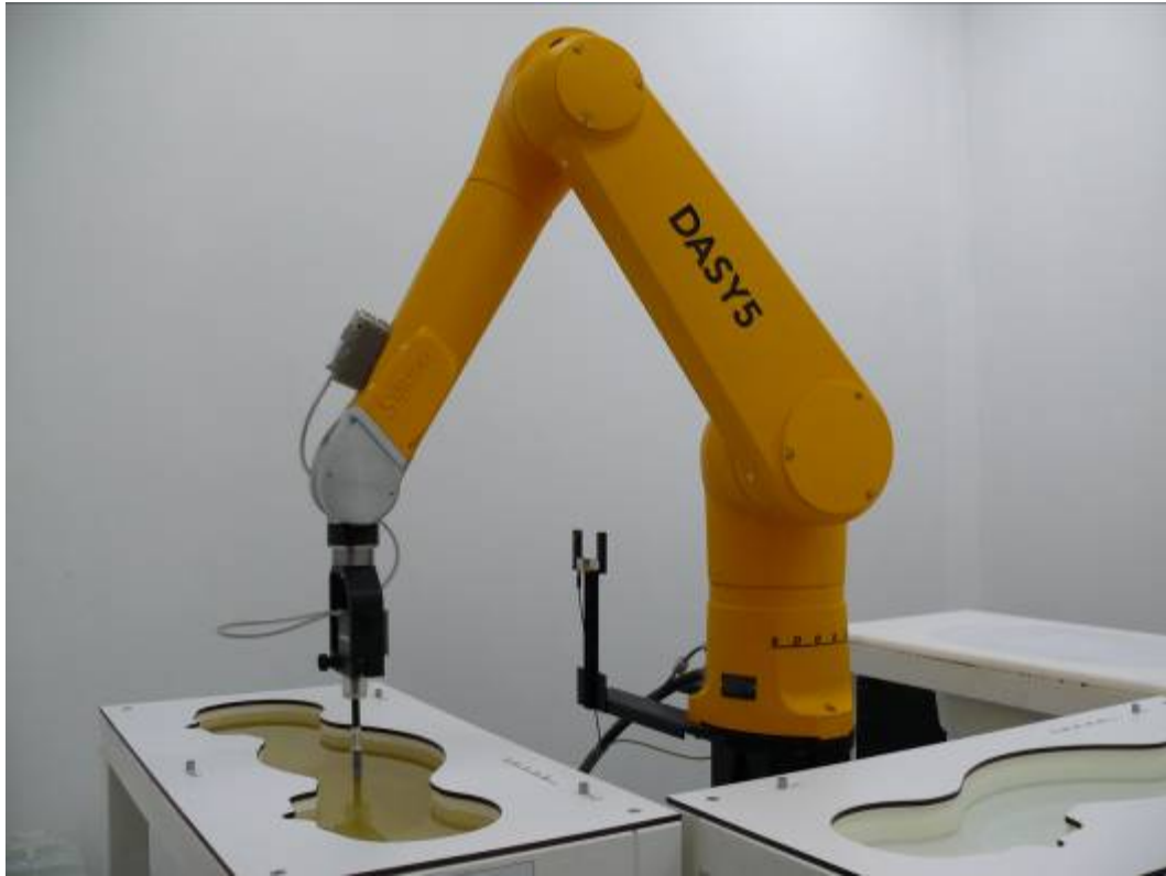
Picture 1: Specific Absorption Rate Test Layout
