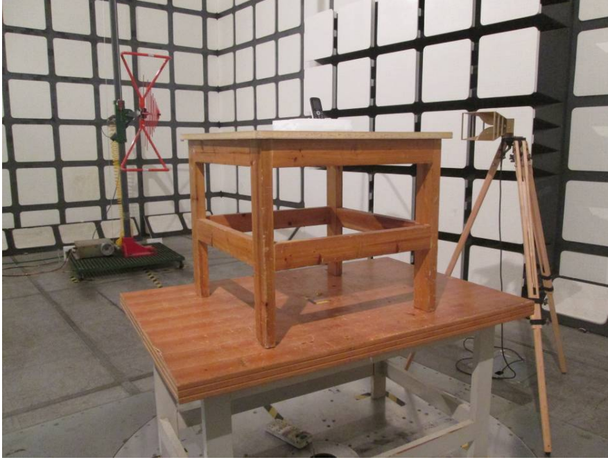
Radiated Emissions Test View (Below 1 GHz)
