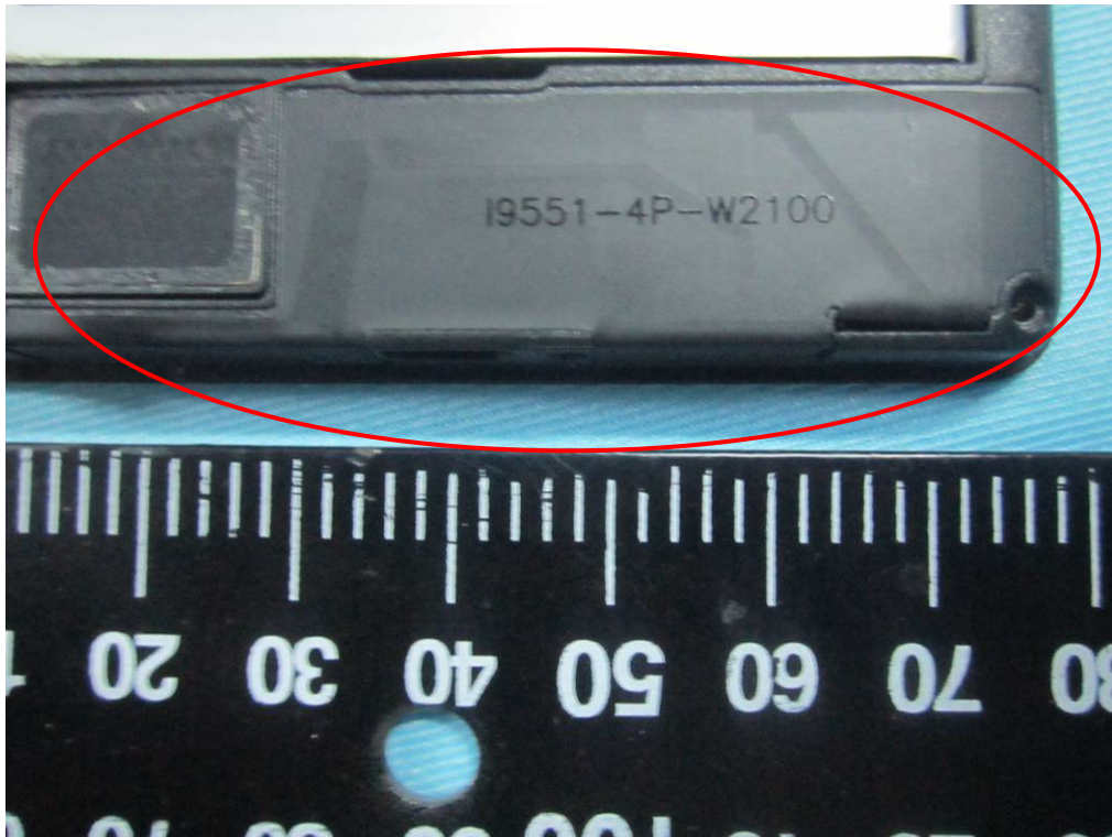
GSM/PCS/UMTS-FDD Antenna View
