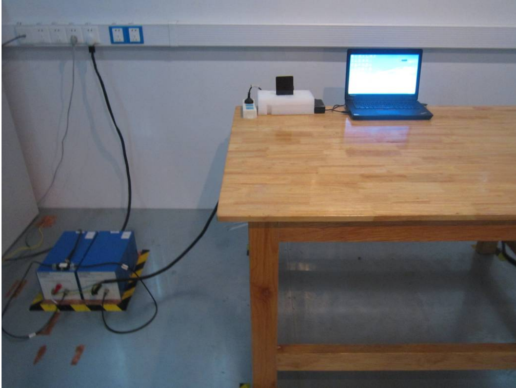
Conducted Emissions Test Setup Front View
