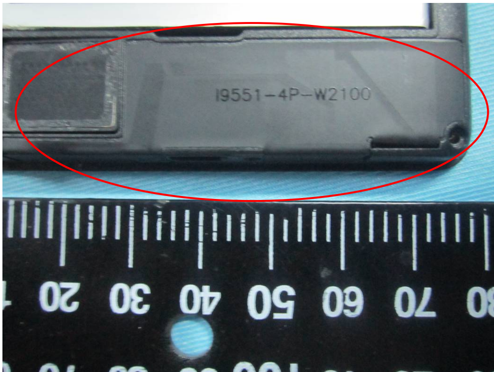
GSM/PCS/UMTS-FDD Antenna View
