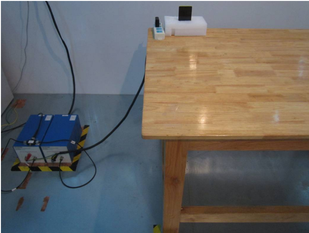
Conducted Emissions Test Setup Front View
