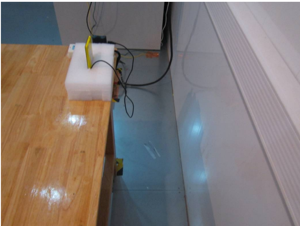
Conducted Emissions Test Setup Side View
