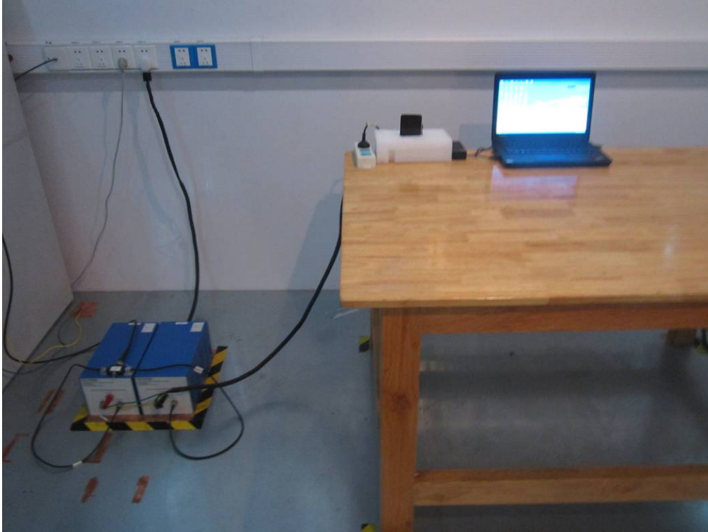
Conducted Emissions Test Setup Front View
