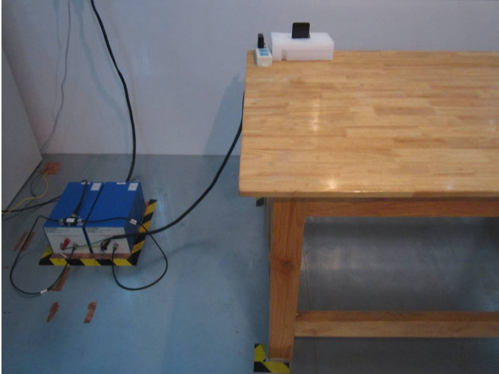
Conducted Emissions Test Setup Front View
