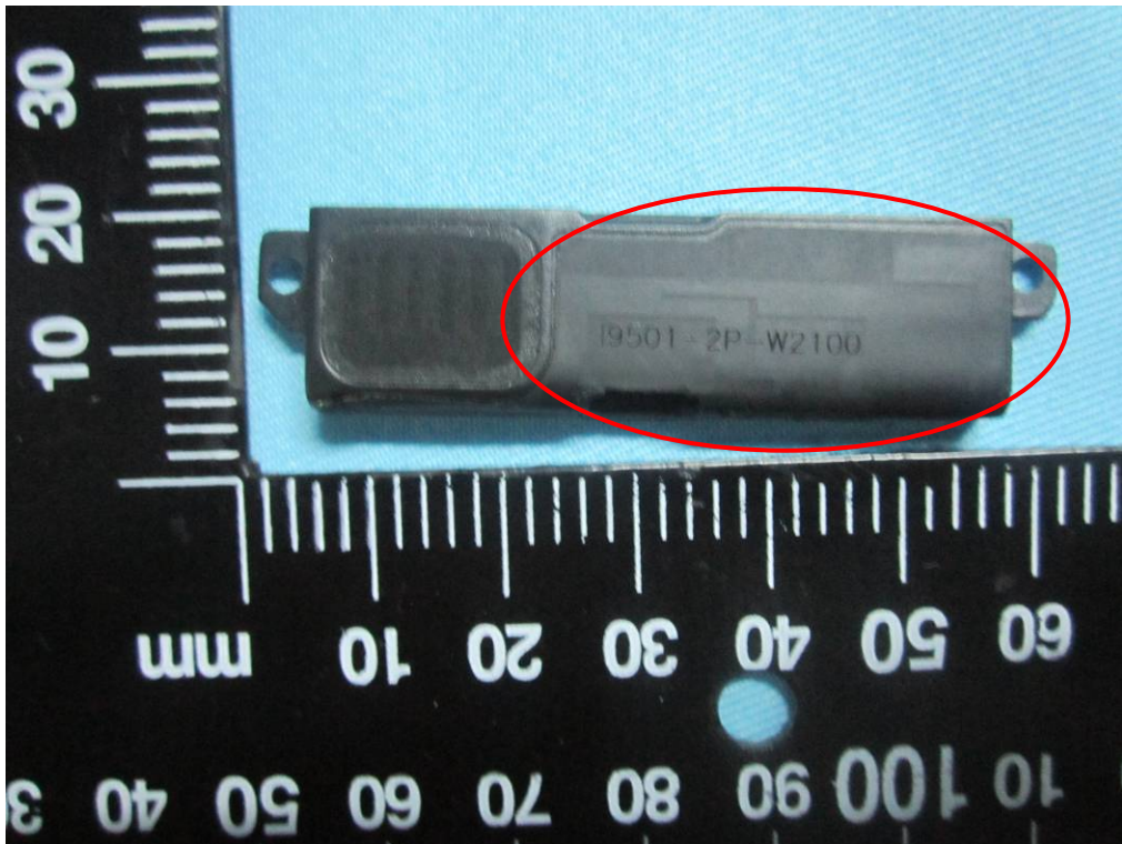
GSM/PCS/UMTS-FDD Antenna View
