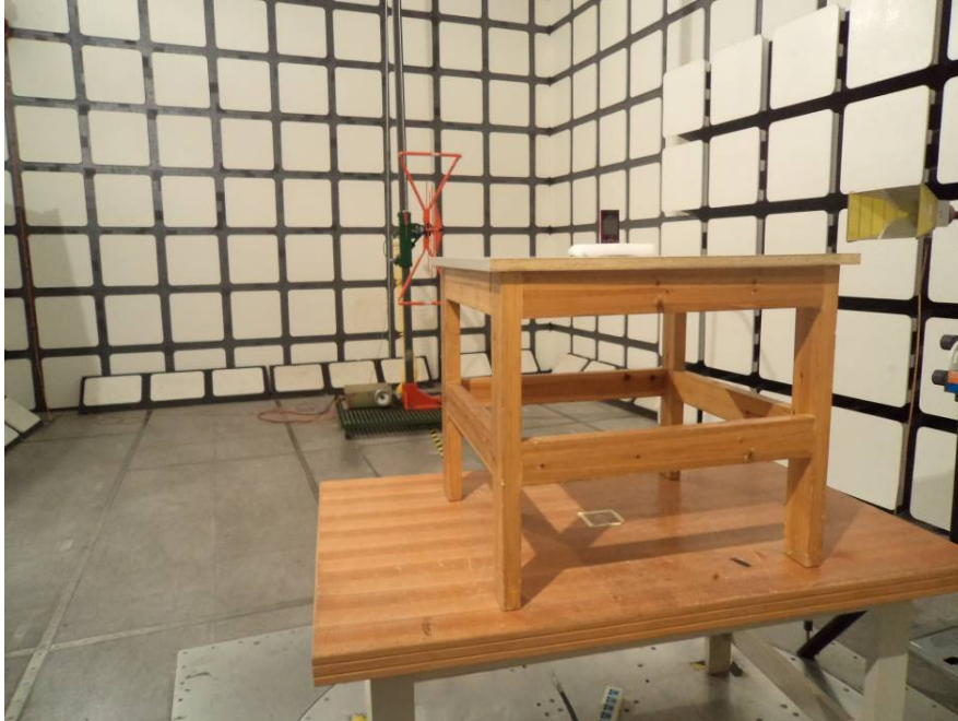
Radiated Emissions Test View (Below 1 GHz)
