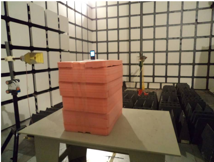
Radiated Emissions Test View (Above 1 GHz)
