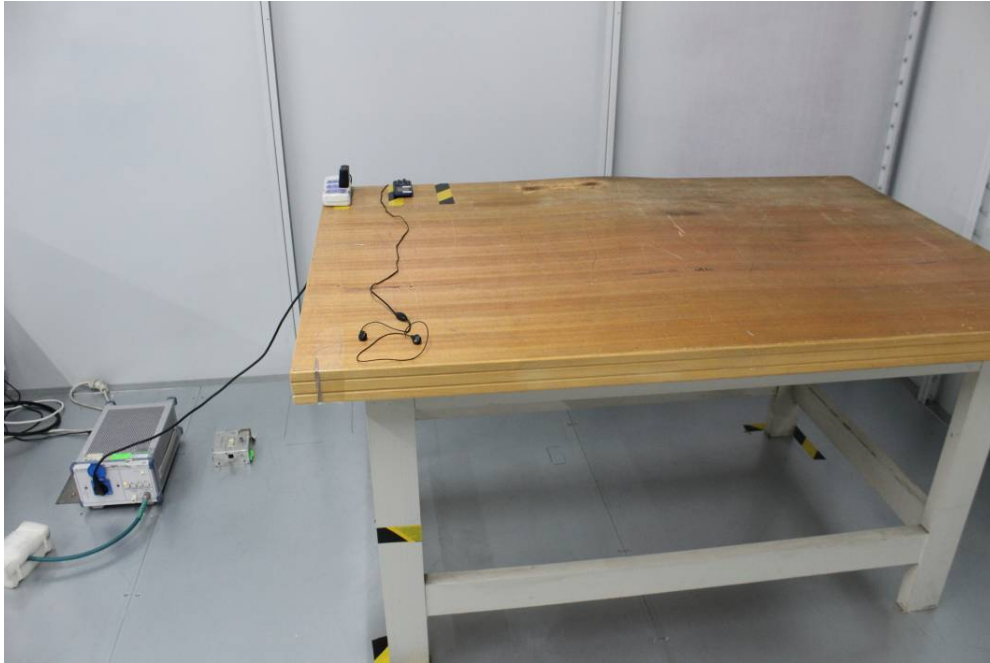
Conducted Emissions - Front View
