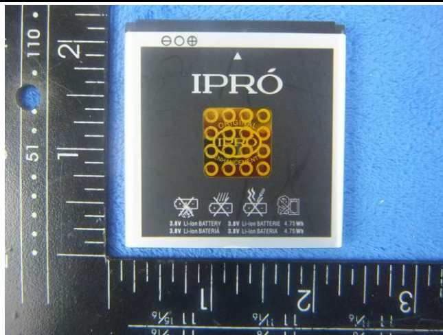
Battery - Top View
