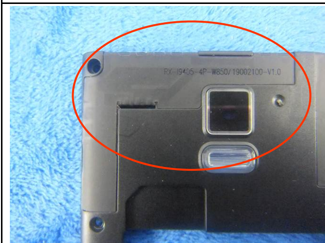
GSM/PCS/UMTS-FDD Antenna View
