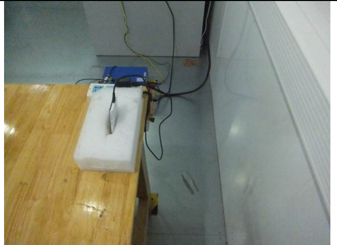
Conducted Emissions Test Setup Side View
