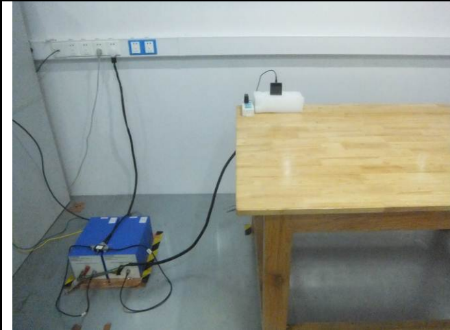
Conducted Emissions Test Setup Front View
