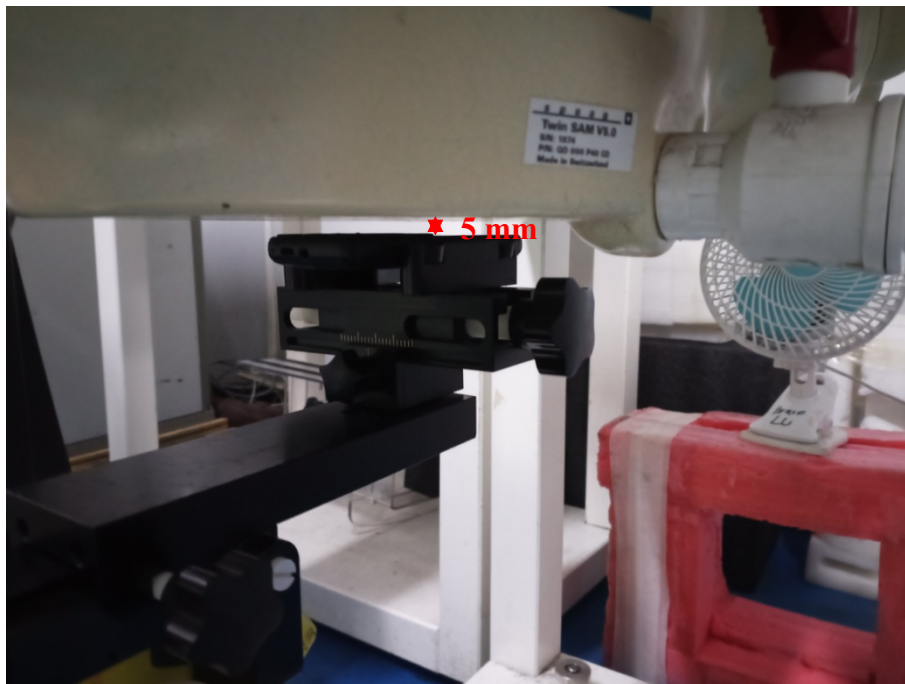
Body (Worn) Front Setup Photo(5mm)
