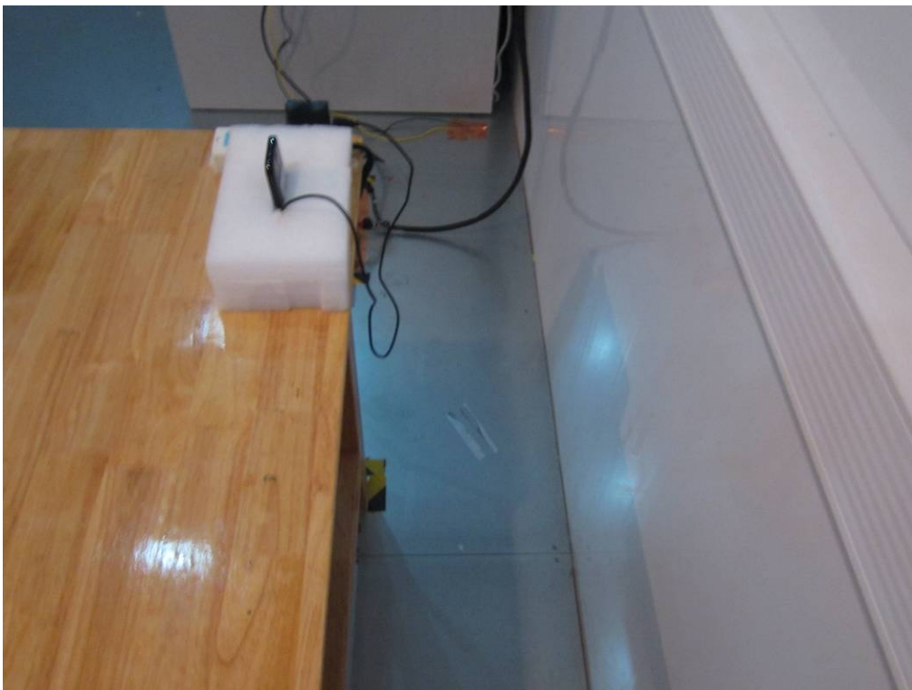
Conducted Emissions Test Setup Side View
