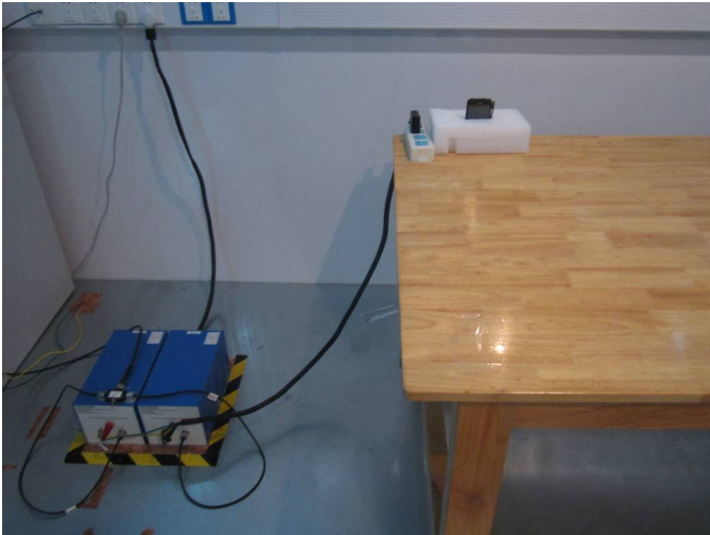
Conducted Emissions Test Setup Front View
