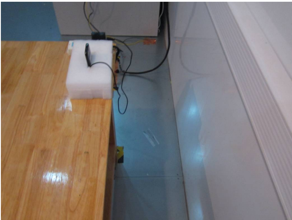
Conducted Emissions Test Setup Side View
