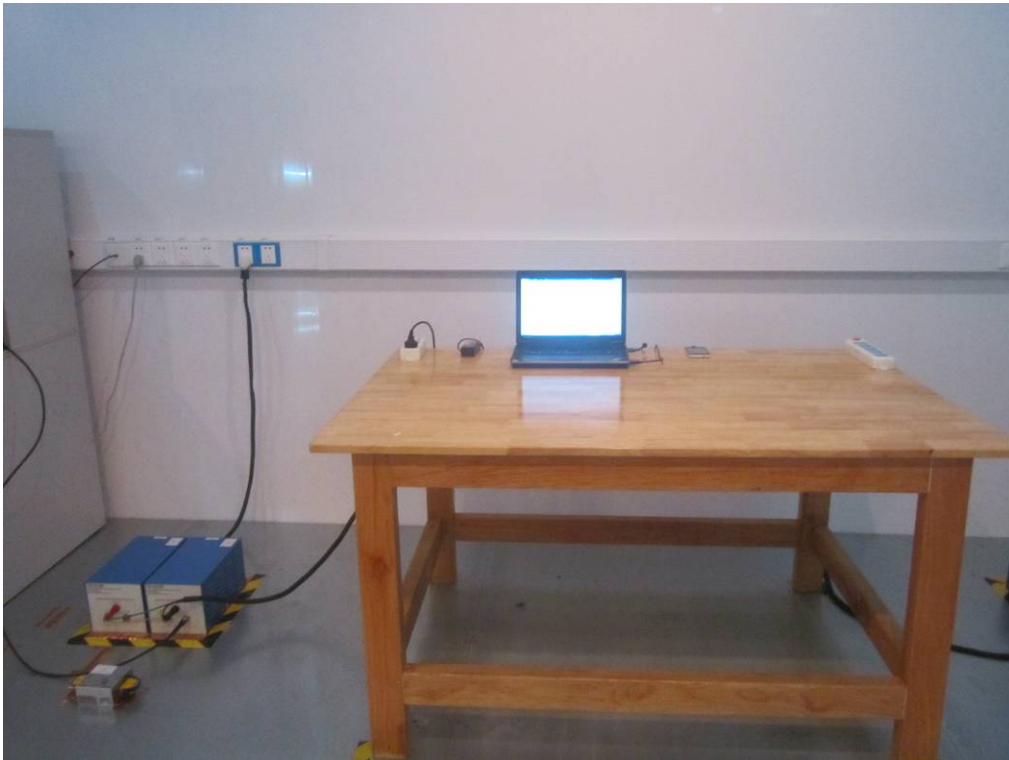
Conducted Emissions Test Setup Front View
