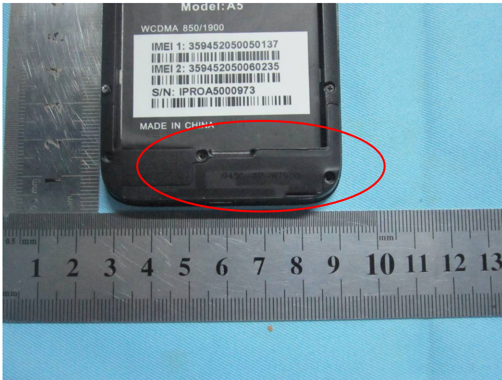
GSM / PCS/ UMTS Antenna View
