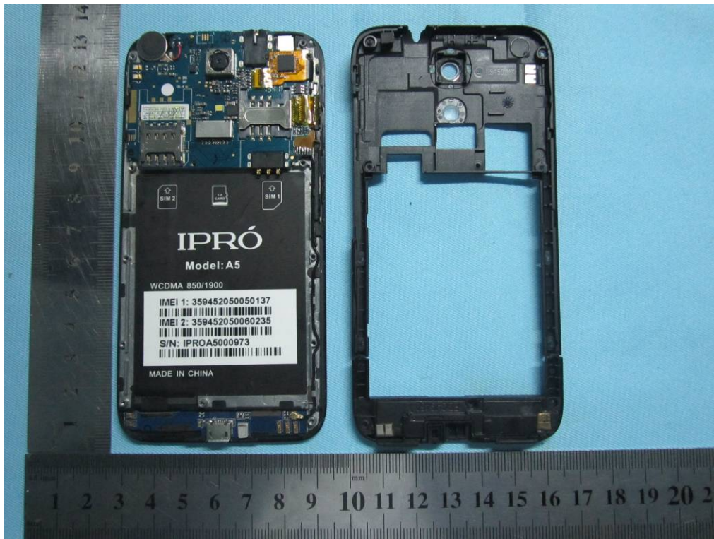
Cover Off - Rear Housing View
