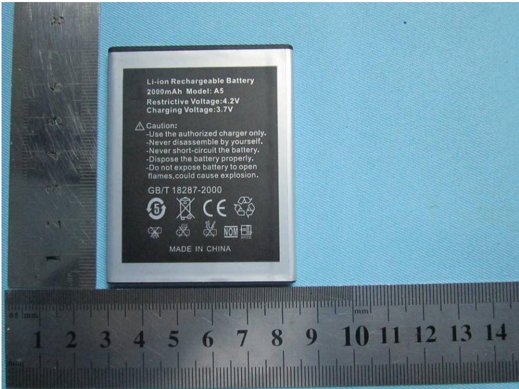
Battery - Top View
