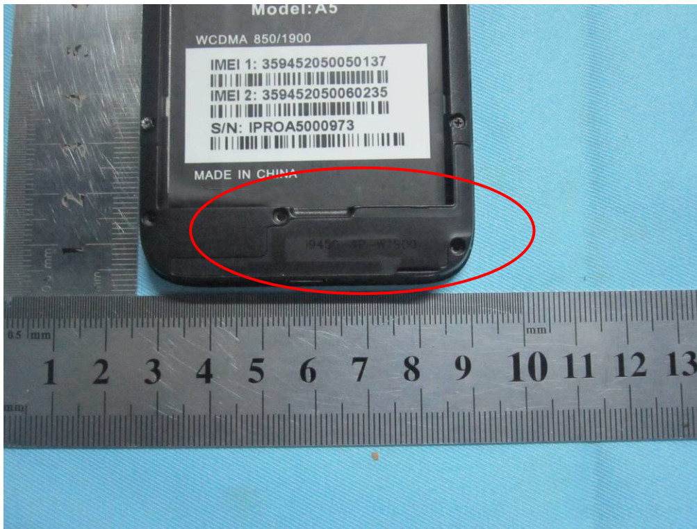
GSM / PCS/ UMTS Antenna View
