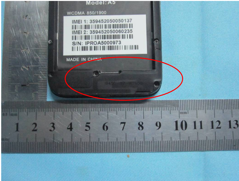
GSM / PCS/ UMTS Antenna View
