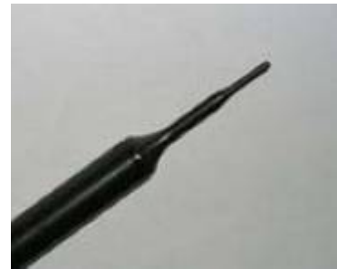
Picture C.2 Near-field Probe
