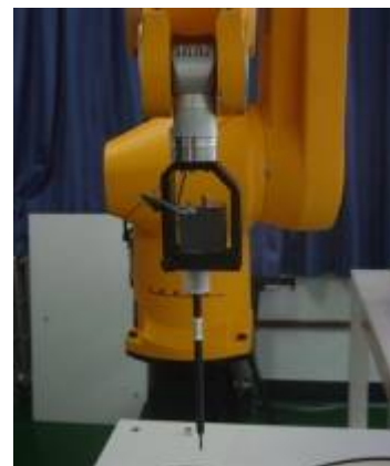
Picture C.3 E-field Probe
