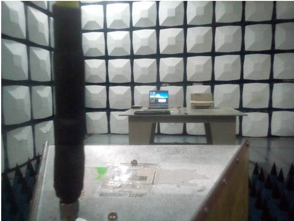
Radiated Emissions Above 1G front View
