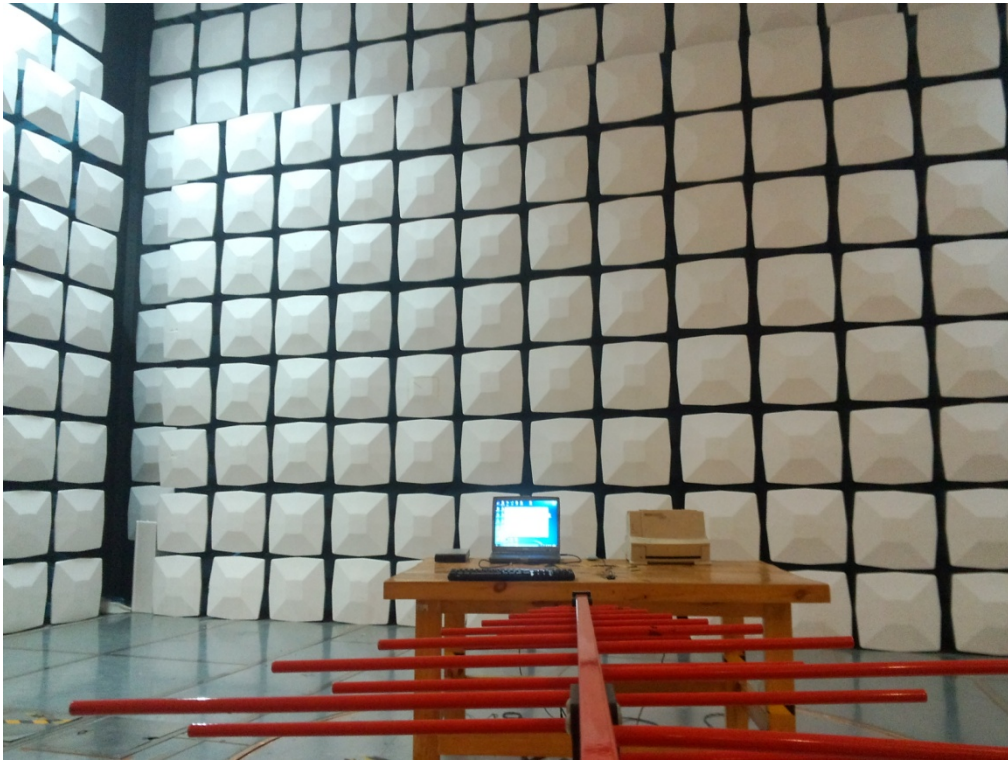
Radiated Emissions Below 1G front View
