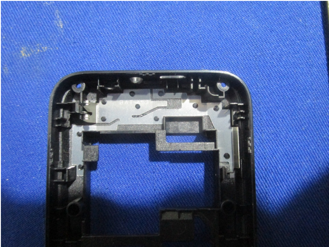
GSM Antenna View
