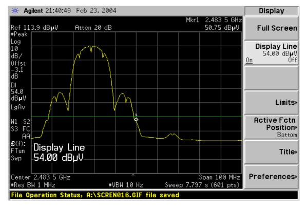
Detector mode: Peak Polarity: Horizontal
