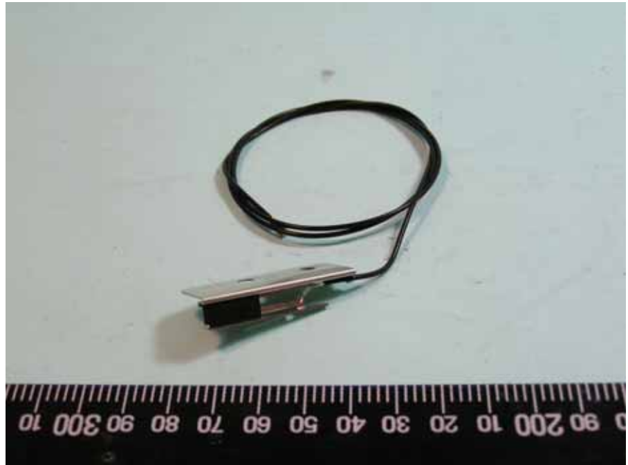
Wistron: Dipole Antenna (W/O cable)-XCC / 2.00dBi
