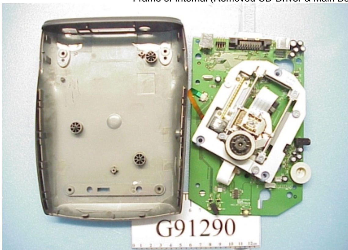
Figure 8 CD-RW DRIVE, M/N: LXR-40122A Frame of Internal (Removed CD-Driver & Main Board)
