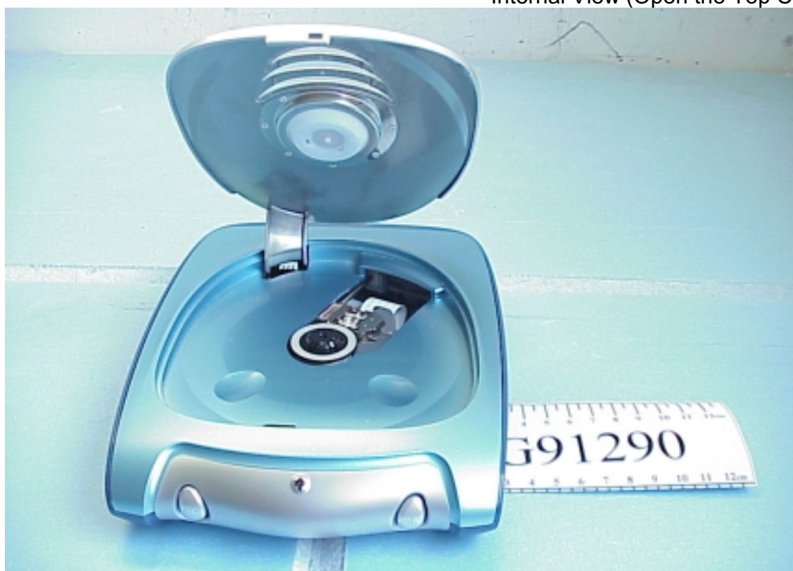
Figure 22 CD-RW DRIVE, M/N: LXR-40122B Internal View (Open the Top Cove)
