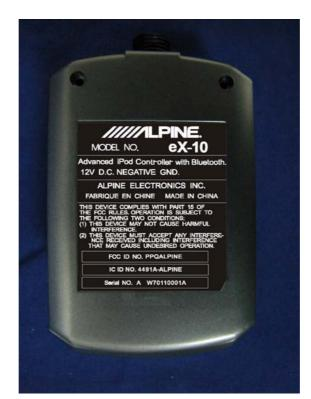
The FCC ID and Label will be placed on the equipment as shown in the photograph below.
