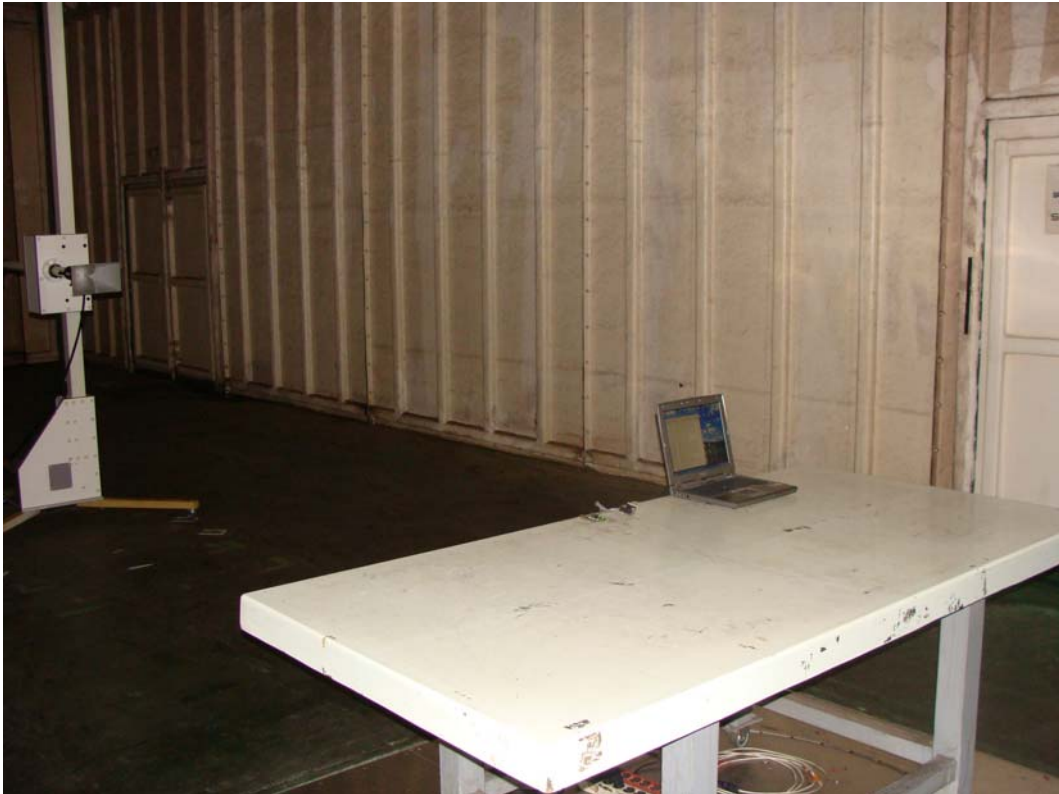
Back View of Radiated Test (Horn) 1-18GHz
