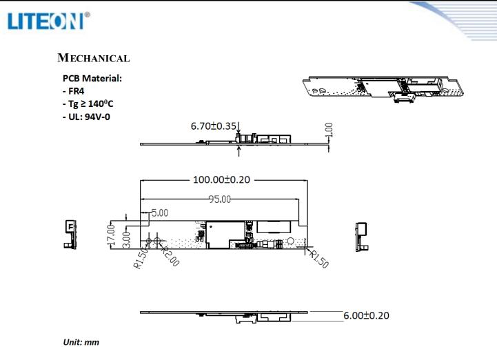
Unit: mm Tolerance: ±0.10mm
