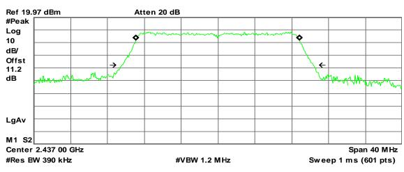
Occupied Bandwidth 17.7964 MHz Occ BW % Fw r 99.00 % x dB -26.00 dB
