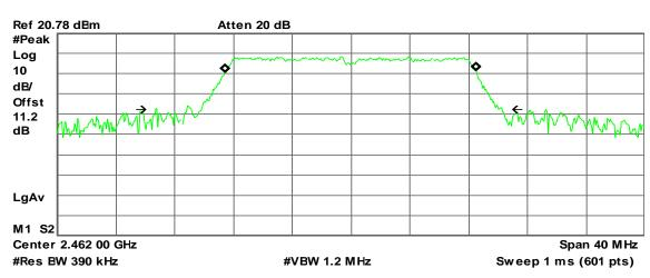
Occupied Bandwidth 17.1331 MHz Occ BW % Fw r 99.00 % x dB -26.00 dB
