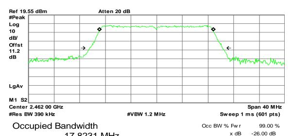
Transmit Freq Error -38.827 kHz x dB Bandw idth 20.699 MHz
