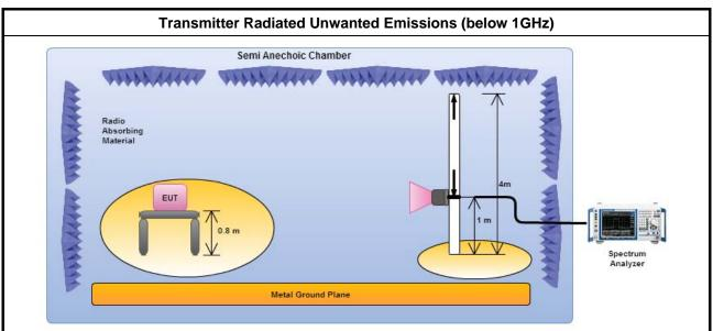
Magnetic field tests shall be performed in the frequency range of 9 kHz to 30 MHz using a calibrated loop antenna. Electric field tests shall be performed in the frequency range of 30 MHz to 1000 MHz using a calibrated bi-log antenna.
