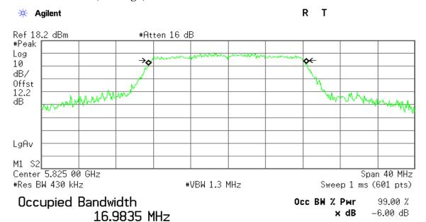
Transmit Freq Error -64.895 kHz x dB Bandwidth 16.276 MHz
