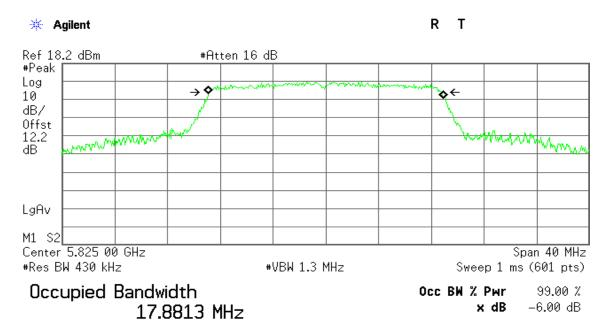
Transmit Freq Error 4.977 kHz x dB Bandwidth 17.705 MHz
