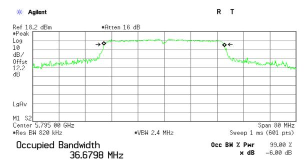
Transmit Freq Error -77.288 kHz x dB Bandwidth 36.136 MHz
