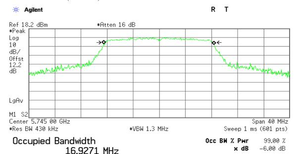
Transmit Freq Error -71.350 kHz x dB Bandwidth 16.498 MHz
