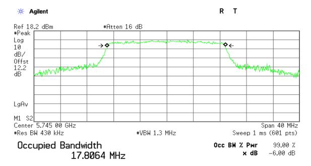
Transmit Freq Error -69.564 kHz x dB Bandwidth 17.633 MHz
