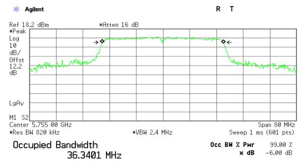
Transmit Freq Error -64.863 kHz x dB Bandwidth 35.944 MHz 6dB Bandwidth (CH High)
