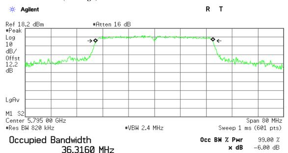
Transmit Freq Error -52.247 kHz x dB Bandwidth 35.963 MHz
