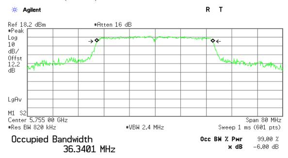
Transmit Freq Error -64.863 kHz x dB Bandwidth 35.944 MHz
