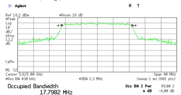
Transmit Freq Error -50.202 kHz x dB Bandwidth 17.577 MHz
