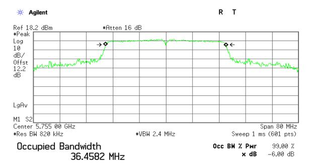
Transmit Freq Error -59.421 kHz x dB Bandwidth 36.051 MHz
