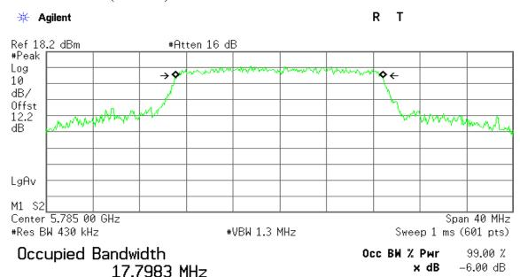
Transmit Freq Error -63.363 kHz x dB Bandwidth 17.616 MHz
