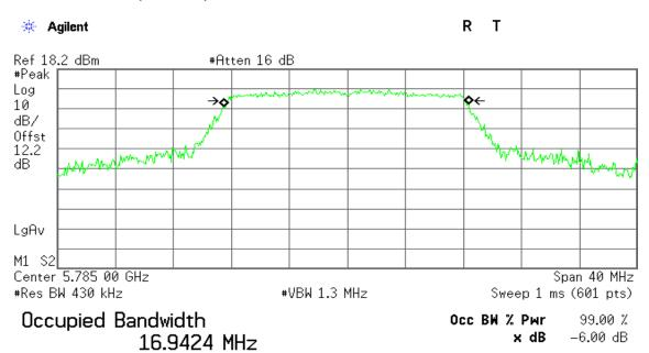
Transmit Freq Error -80.626 kHz x dB Bandwidth 16.392 MHz
