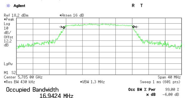
Transmit Freq Error -80.626 kHz x dB Bandwidth 16.392 MHz
