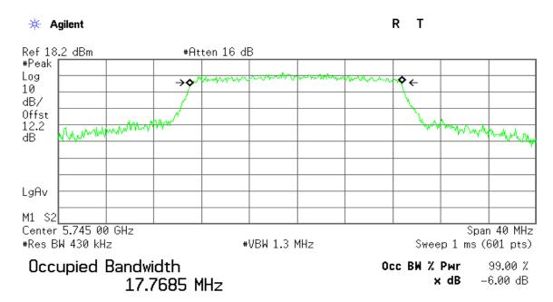
Transmit Freq Error -91.622 kHz x dB Bandwidth 17.535 MHz
