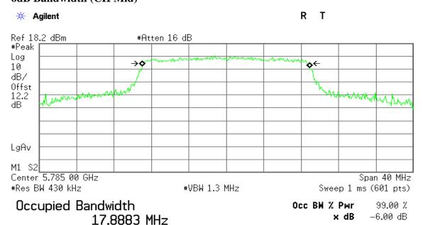
Transmit Freq Error -39.982 kHz x dB Bandwidth 17.479 MHz
