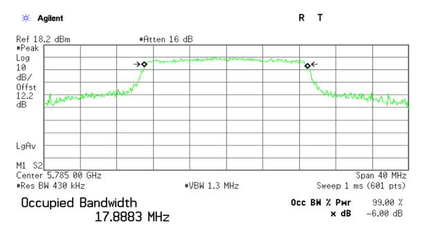
Transmit Freq Error -39.982 kHz x dB Bandwidth 17.479 MHz
