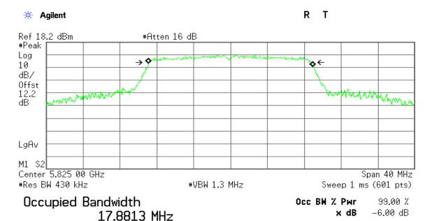
Transmit Freq Error 4.977 kHz x dB Bandwidth 17.705 MHz
