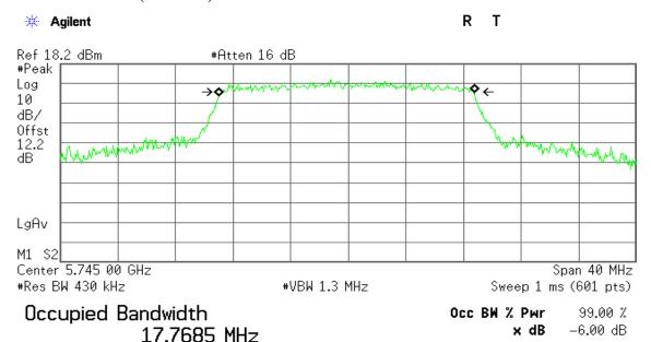
Transmit Freq Error -91.622 kHz x dB Bandwidth 17.535 MHz
