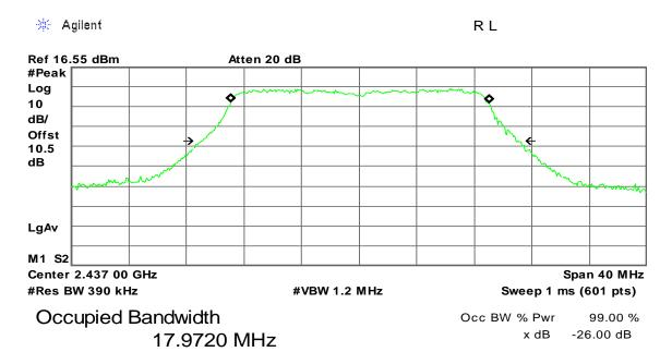
Transmit Freq Error 48.093 kHz x dB Bandwidth 21.772 MHz
