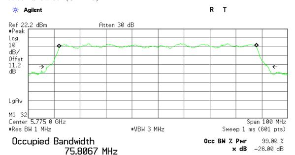
Transmit Freq Error -16.654 kHz x dB Bandwidth 84.902 MHz
