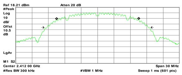
Occupied Bandwidth 15.0504 MHz Occ BW % Pwr 99.00 % x dB -26.00 dB
