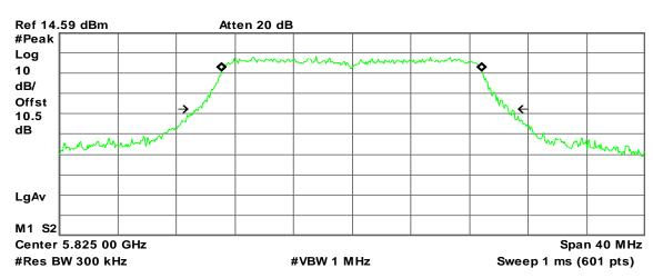
Occupied Bandwidth 17.8067 MHz Occ BW % Pwr 99.00 % x dB -26.00 dB
