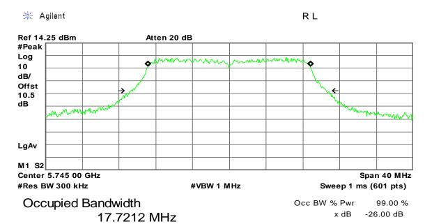
Transmit Freq Error -24.211 kHz x dB Bandwidth 21.261 MHz
