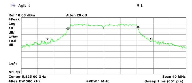
Occupied Bandwidth 16.9752 MHz Occ BW % Pwr 99.00 % x dB -26.00 dB
