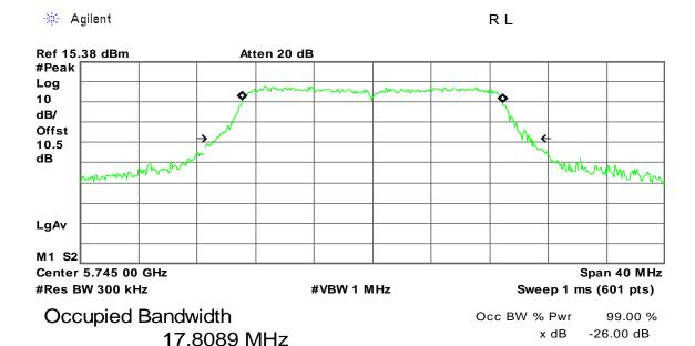
Transmit Freq Error -2.715 kHz x dB Bandwidth 21.552 MHz
