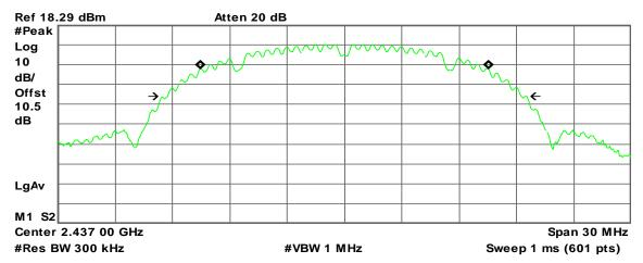
Occupied Bandwidth 15.0559 MHz Occ BW % Pwr 99.00 % x dB -26.00 dB
