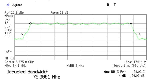
Transmit Freq Error -12.593 kHz x dB Bandwidth 84.590 MHz
