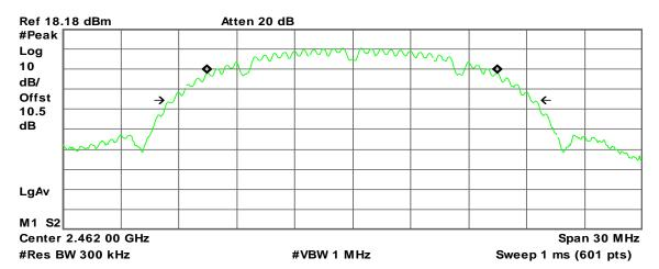
Occupied Bandwidth 15.0506 MHz Occ BW % Pwr 99.00 % x dB -26.00 dB
