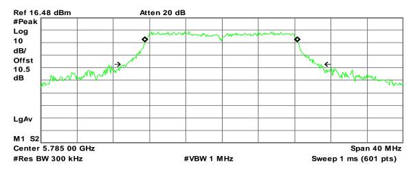
Occupied Bandwidth 16.8416 MHz Occ BW % Pwr 99.00 % x dB -26.00 dB
