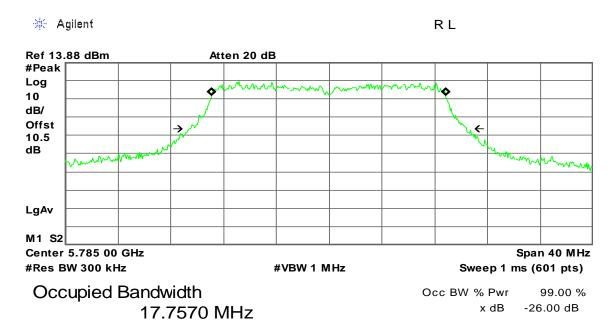
Transmit Freq Error -30.235 kHz x dB Bandwidth 20.910 MHz
