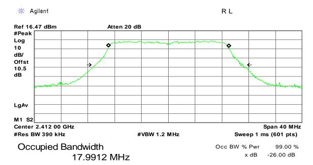
Transmit Freq Error 69.938 kHz x dB Bandwidth 21.973 MHz
