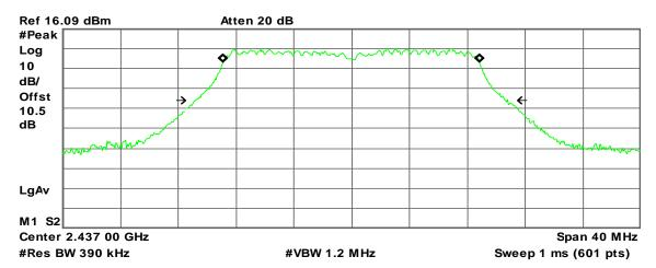
Occupied Bandwidth 17.7845 MHz Occ BW % Pwr 99.00 % x dB -26.00 dB
