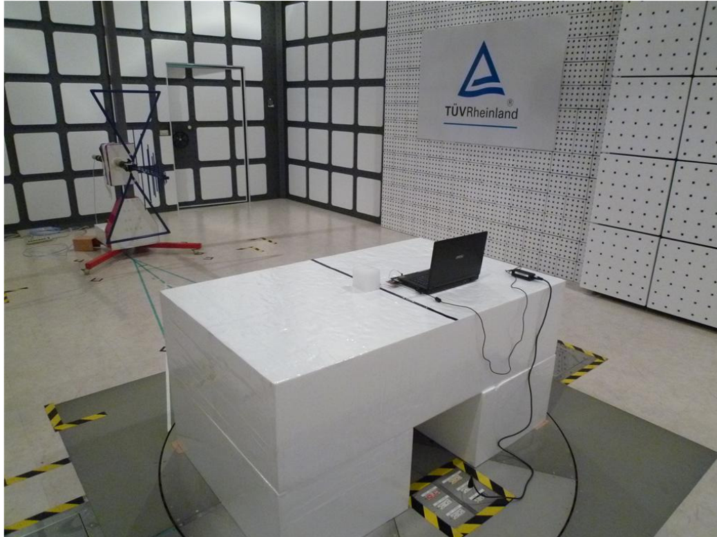
Photograph 2: Set-up for Spurious Emissions (Back View 1)
