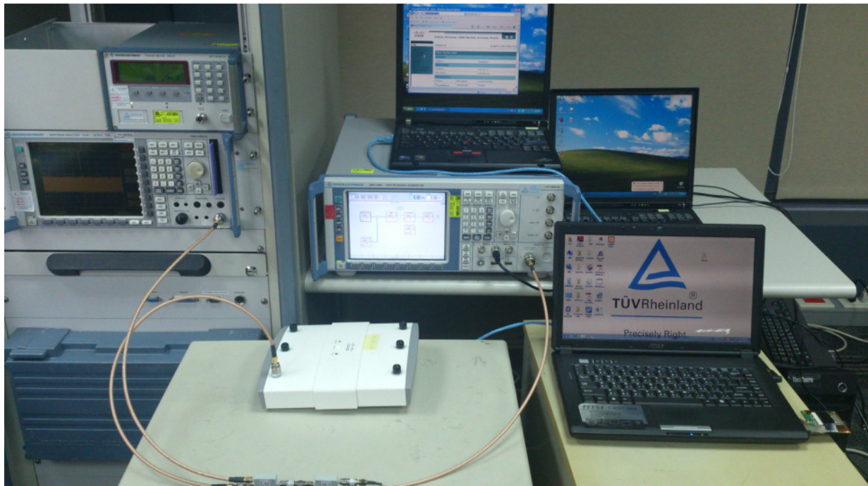
Photograph 2: Set-up for DFS testing
