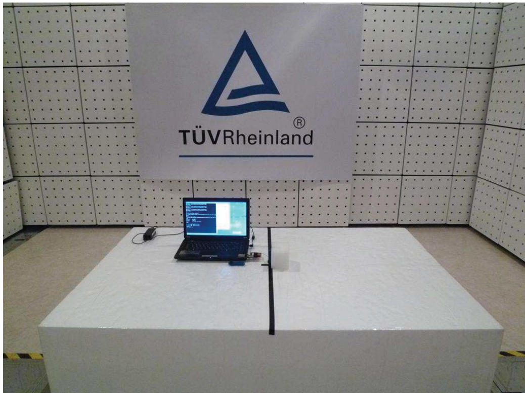
Photograph 1: Set-up for Spurious Emissions (Front View)
