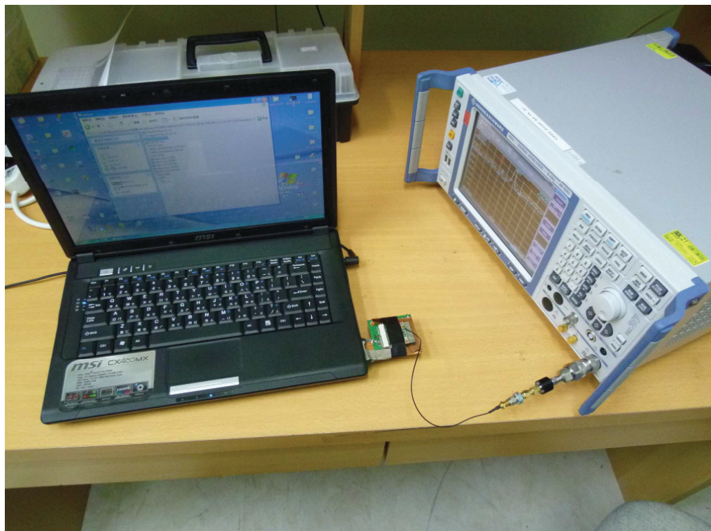
Photograph 4: Set-up for Conducted testing
