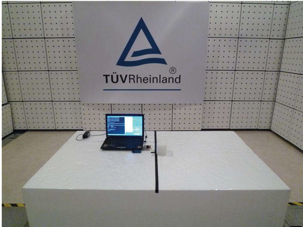
Photograph 1: Set-up for Spurious Emissions (Front View)
