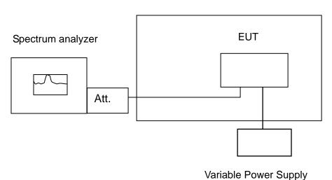
Remark: Measurement setup for testing on Antenna connector
