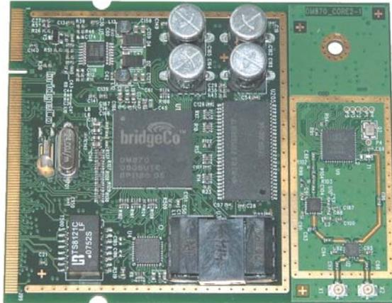
The DM870 Core-2 module is a single-board networked media player module, based on BridgeCo's DM870 media processor, and enables fast product developments with ethernet, WiFi and USB connectivity. The module connects to standard legacy components in various audio, video/LCD and control formats. It runs from a single 5V power supply and creates all the necessary voltages on the module. A stabilized 3.3V power is provided to the main board, to allow for further system cost reduction.
