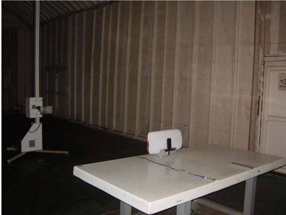
Front View of Radiated Test (Horn)
