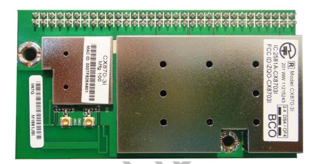
3.4 Production Module with 64-pin Connector Option – Side View
