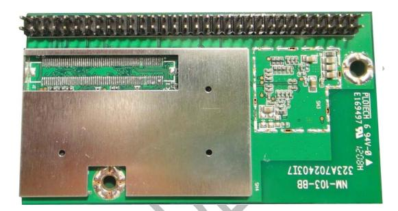
3.6.2 Including J2 High Density 120-pin connector – Bottom View
