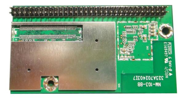
3.6.2 Including J2 High Density 120-pin connector – Bottom View
