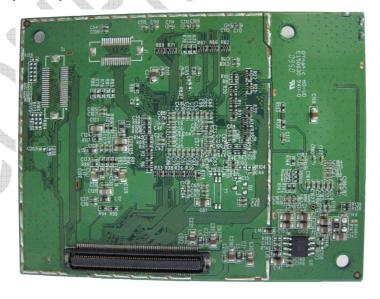
Versions with no bottom shield and no LCD connector.
