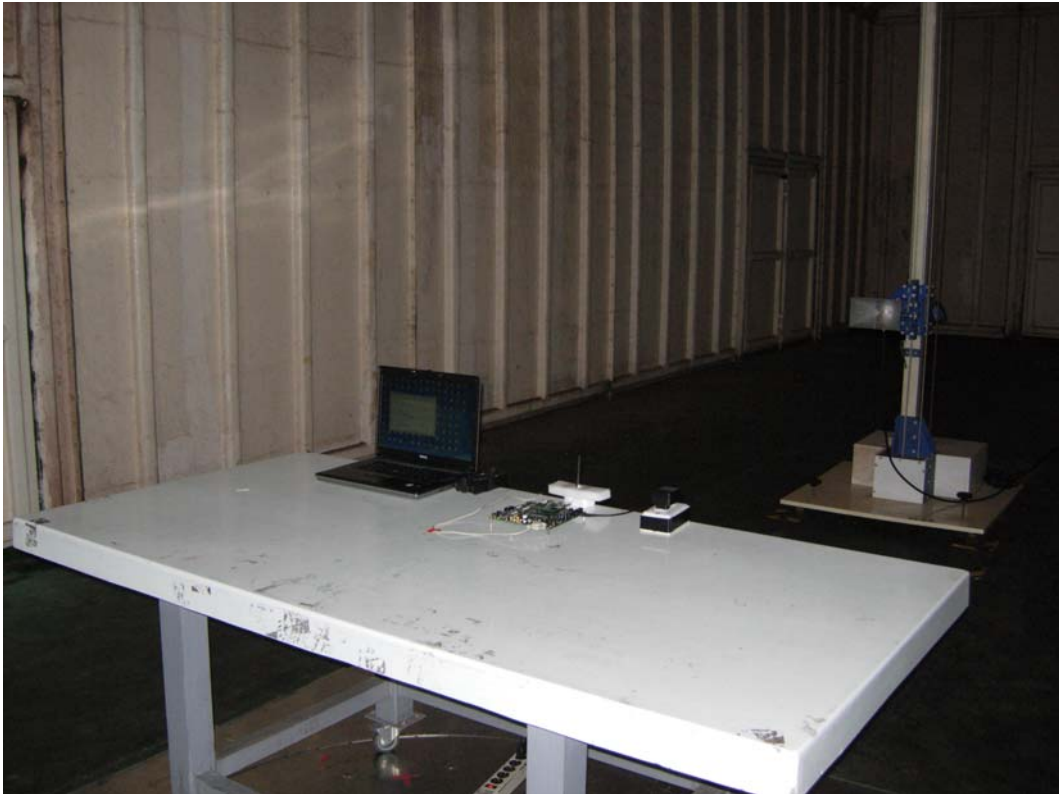
Back View of Radiated Test (Horn)
