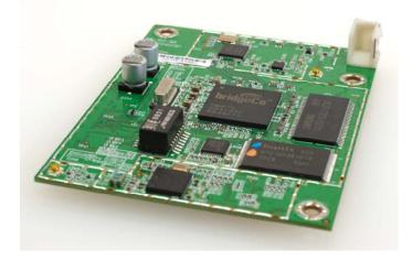
Complete audio networking system on a small module
