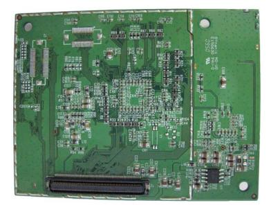
Versions with no bottom shield and no LCD connector.
