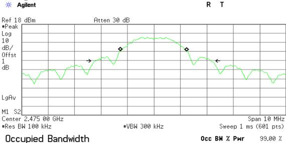
Transmit Freq Error -14.750 kHz x dB Bandwidth 4.374 MHz
