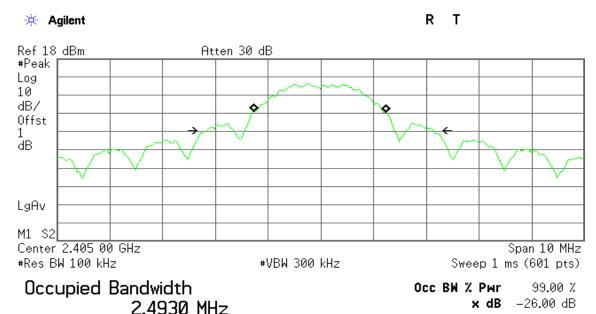
Transmit Freq Error -19.034 kHz x dB Bandwidth 4.329 MHz
